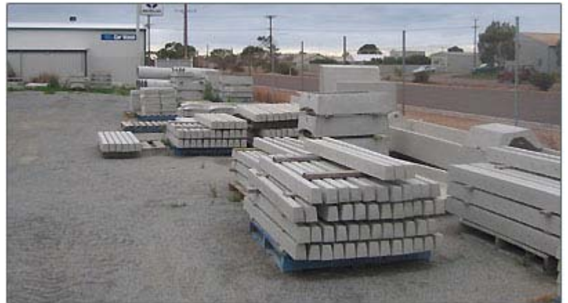
Stockpile of gate post strainers
